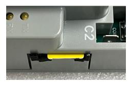
When properly inserted and latched approximately 2mm of the SIM will be exposed.
