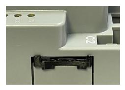
The SIM slot is located on the right side of the AVW400 monitor near the three LEDs labeled TX, RX, and S. The Type II Cellular Module is designed to accept the SIM card inserted directly into the slot. There is no tray to hold the SIM with the Type II module.
