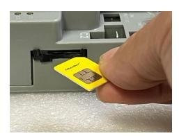
Hold the SIM with the gold contacts facing up and the notched corner facing away from your hand. Slide the SIM into the SIM slot and push in until it stops. A click will be heard and the SIM should be securely held in place.
