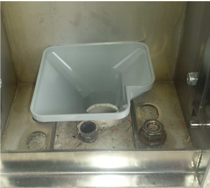
Coin chute installed in a bolt on pedestal.
