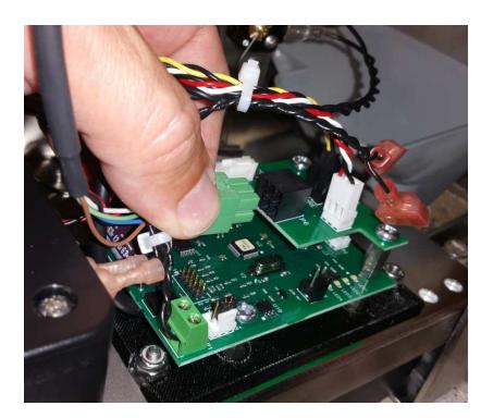
Terminate power supply cable (ASY0000359-02) using included terminals. Plug power supply cable (ASY0000359-02) into power supply adaptor (WICA000382).
